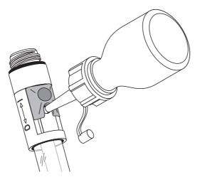
**Cleaning** Remove water-soluble contamination by rinsing with deionized water. Remove other contamination as follows:
