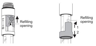
• Remove the watering cap from the electrode tip. Possible salt deposits in the area of the watering cap do not affect the measuring characteristics and can easily be removed with deionized water.
