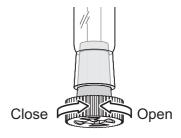
• Carefully and using little power close the junction until the contact between the rough ground surfaces can be noticed as a resistance. The electrode is now ready to measure.
